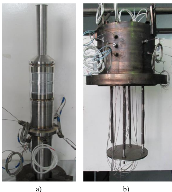
Figure 4 – Experimental Equipment for Researches: Rods Guide Tube Mock-Up (a) and Device Designed for Corium Cooling Efficiency Study (b)
