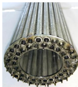
Assembly of Model Fuel Elements with Uranium Dioxide Pellets
