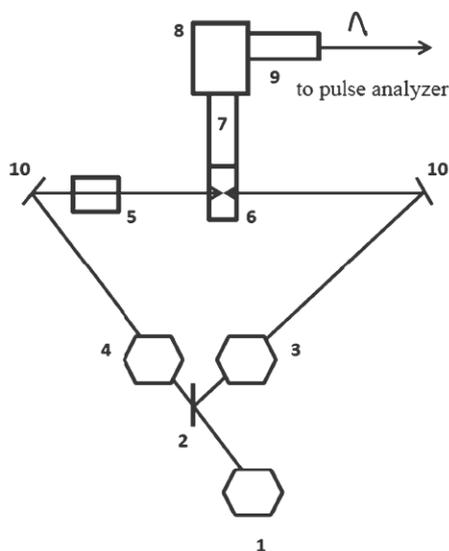
**Fig.8** Scheme of the experimental set up: (1) nitrogen laser OBB-1010, (2) beam splitter, (3) dye laser OBB-1011, (4) dye laser OBB-1012, (5) optical delay line OPD-1, (6) cuvette with solution, (7) optical fiber, (8) monochromator DMR-4, (9) photomultiplier, (10) mirror.
