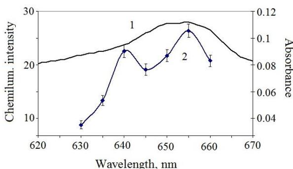
**Fig. 11** (1) The absorption spectrum of Pu(IV) in solution. (2) Chemiluminescence excitation spectrum for the luminol+Pu(IV)+CsF solution using the two-step one-color scheme.
