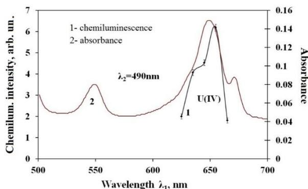
**Fig. 10** (1) Spectrum of chemiluminescence excitation by the scheme two step-two color in luminol + U(IV) solution. (2) Absorption spectrum of U(IV) in aqueous HCl solution.
