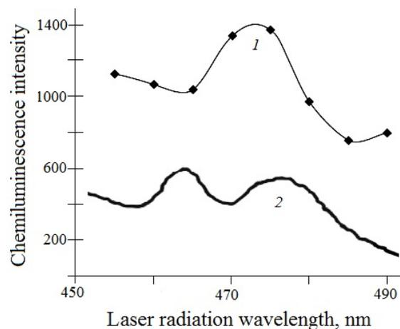
**Fig.9** (1) Spectrum of chemiluminescence excitation by the scheme two step-one color in luminol +  $\text{Sm}(\text{III})$  solution. (2) Absorption spectrum of  $\text{Sm}^{3+}$ .
