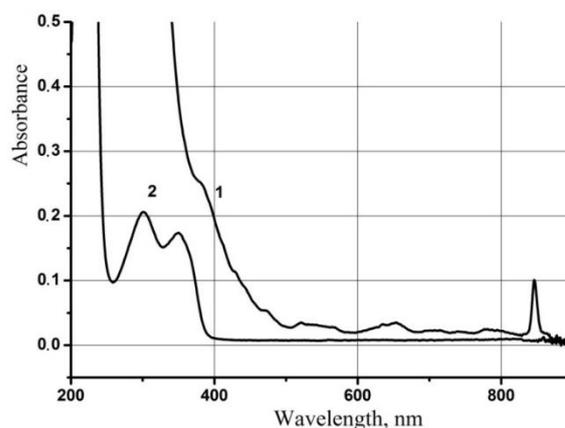
**Fig. 7** Absorption spectra: 1 –  $\text{PuO}_2^{2+}$  (0.003 M) in solution 42%  $\text{CsF} + \text{H}_2\text{O}$ ; 2 – luminol [0.001 M] in solution 42%  $\text{CsF} + \text{H}_2\text{O}$ , pH 10.5.
