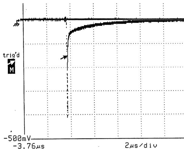
**Fig.1** Time dependence of the uranyl luminescence in a 4.5 M  $H_2SO_4$  solution. Start is a nitrogen laser pulse. The short-lived background luminescence is clearly seen, as well as the relatively long-lived uranyl luminescence. The background luminescence can be significantly suppressed by measuring the luminescence with a delay of several  $\mu s$  after laser pulse.
