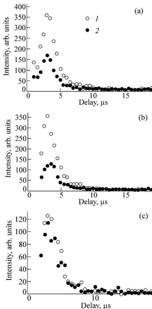
**Fig.4** Kinetics of luminol luminescence at the wavelength 459 nm in 42% solution of CsF in  $\text{H}_2\text{O}$ . pH: (a) 8.19. (b) 9.86. (c) 11.85. (1) - without uranium and (2) 0.009 M of  $\text{UO}_2^{2+}$ . Luminol concentration  $10^{-4}$ . Gate time 1  $\mu\text{s}$ .
