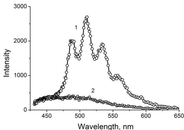
**Fig.3** Photoluminescence (1) of  $UO_2F_5^{3-} [0.005M]$  ( $\circ$ ) in  $CsF(42\%) + H_2O +$  luminol ( $10^{-4} M$ ), and (2) luminol  $10^{-4} M$  ( $\square$ ) in  $CsF(42\%) + H_2O$ , pH 10.07. Excitation by pulsed (10 ns) nitrogen laser. Delay time 2  $\mu s$ . Gate time 100  $\mu s$ .
