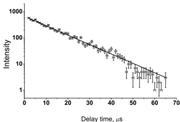
**Fig.2** Photoluminescence of  $UO_2F_5^{3-}$  in  $\{H_2O + CsF [42\%]\}$  solution, pH 9.0. Excitation by nitrogen pulse (10 ns) laser. Registration at  $\lambda=520$  nm,  $\delta\lambda=9$  nm. Gate time 1  $\mu s$ . 200 laser pulses per channel were made. Laser beam diameter 5 mm, power in laser pulse 15 kW. Luminescence lifetime  $\tau = 12.08 \pm 0.25$   $\mu s$ .
