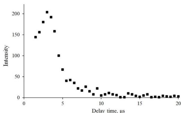
**Fig. 5** Kinetic curve of luminol chemiluminescence induced by excitation of plutonyl in solution.
