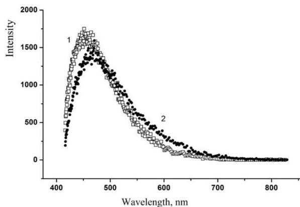
**Fig. 6** Photoluminescence of  $\text{PuO}_2\text{F}_3^{3-}$  [0.001M] + luminol  $10^{-4}\text{M}$  (●) in  $\text{CsF}(42\%) + \text{H}_2\text{O}$  (2), and (1) luminol  $10^{-4}\text{M}$  (□) in  $\text{CsF}(42\%) + \text{H}_2\text{O}$ , pH 8.5. Excitation by pulsed (10ns) nitrogen laser. 200 laser pulse were made per channel at spectrum measurement, laser beam diameter 5 mm, power in laser pulse 15 kW. Delay time 2  $\mu\text{s}$ . Gate time 50  $\mu\text{s}$ .
