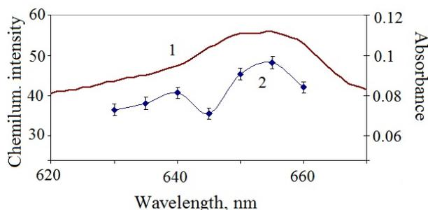
**Fig.12** Comparison of (1) the absorption spectrum of Pu(IV) and (2) the intensity of chemiluminescence at various wavelengths of radiation generated by the OBB-1012 dye laser (two-step two-color scheme).
