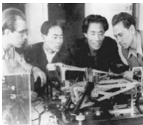
Picture 1. General view of the photo-paper electric magnetic ground motion recorder
