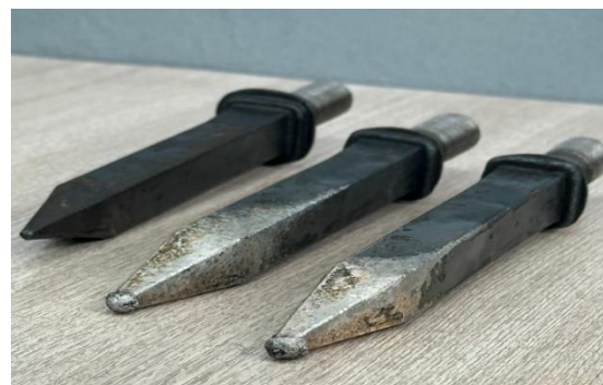
Figure 6. Visual appearance of harrow teeth: initial (far left) and after EPH (sample 1 and 2)
