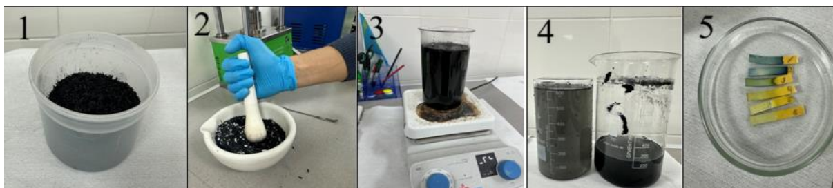
Figure 2. Carbonized RH (1); Mixing with KOH activator (2); The desilification process using boiling and neutralizing pH (~7) (3–5)
