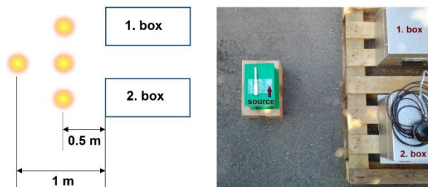
Fig. 2. Point source positions (to the left, not to scale), measurement with a source located centrally at 50 cm (to the right)
