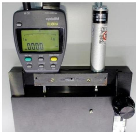
a) device for calibration of linear displacement sensors
