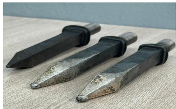
Figure 6. Visual appearance of harrow teeth: initial (far left) and after EPH (sample 1 and 2)
