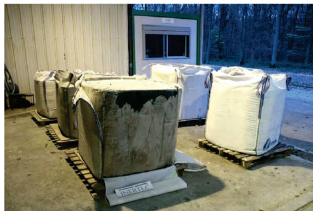
Figure 6. Appearance of concrete blocks produced from processed sodium from the Superphénix reactor
