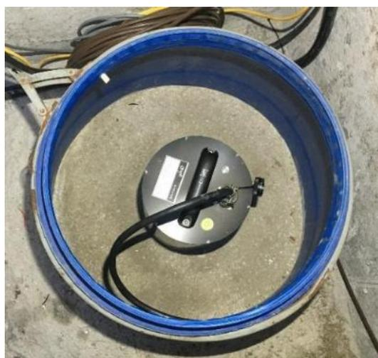
a) seismometer inside the vault
